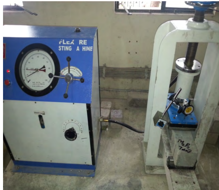
Fig 3. Experimental setup for flexural test
