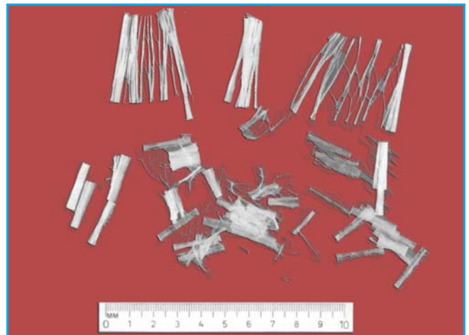
FIGURE 5: Examples of monofilament and fibrillated micro synthetic fibres. (Source: Advanced Concrete Technology edited by Newman and Choo).
