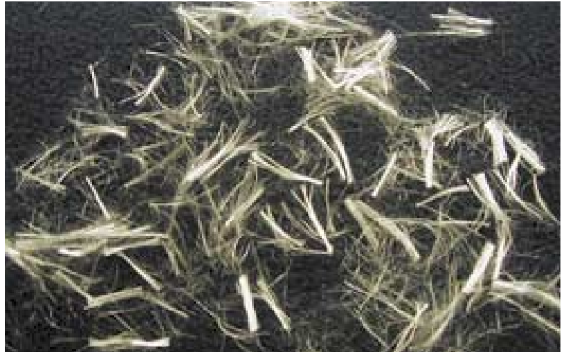
Figure 1: Monofilament polypropylene fibres.
