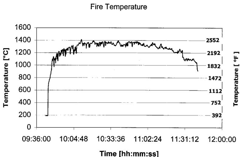
Figure 2: Furnace temperature versus time curve (RWS Curve).
