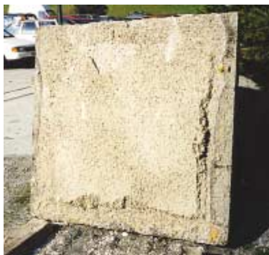
Figure 6: Steel + micro PP fiber shotcrete panel after 2-h fire test.
