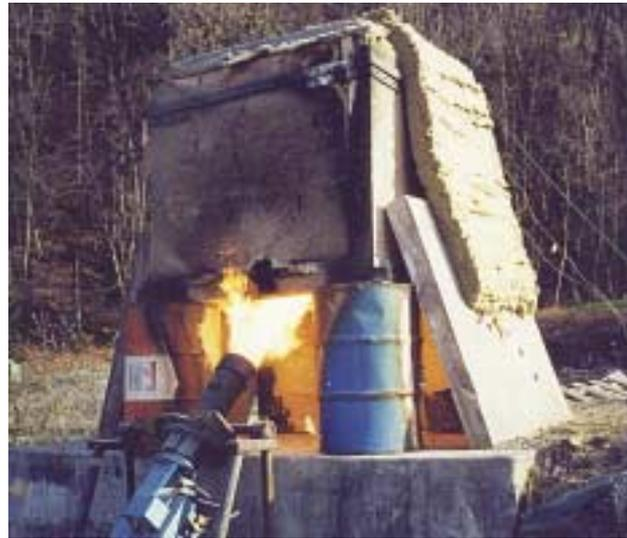
Figure 3: Hagerbach hydrocarbon-fueled fire furnace setup.
