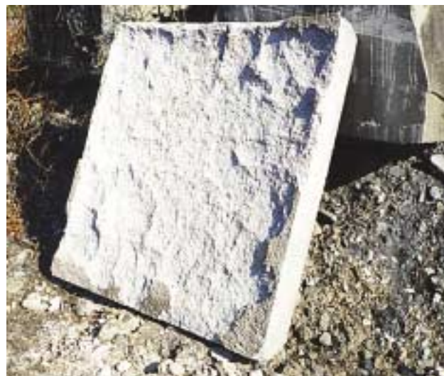
Figure 4: Nonfibrous mesh reinforced panel: 15-min fire test.
