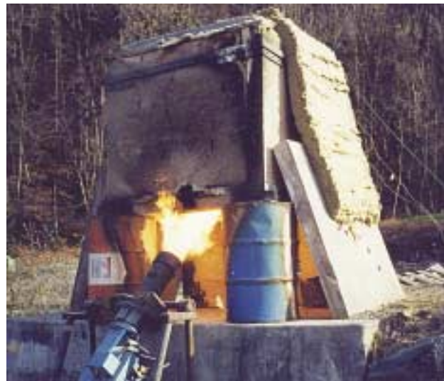
Figure 3: Hagerbach hydrocarbon-fueled fire furnace setup.
