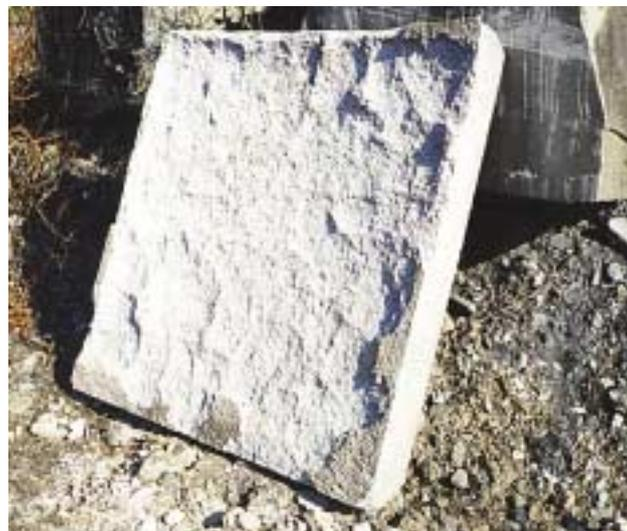
Figure 4: Nonfibrous mesh reinforced panel: 15-min fire test.
