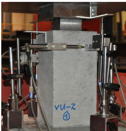
Fig. 2 Test set-up for concentrated loading tests (left) and positioning of the specimen for centric and eccentric loading (right)
