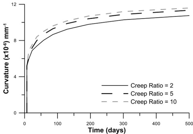
**Fig. 13** Effect of fibre creep on the time-varying curvature ( $A_{s1} = A_{s2} = 1000 \text{ mm}^2$ ,  $\rho_f = 3 \text{ kg/m}^3$ ,  $N_e = -300 \text{ kN}$  and  $M_e = 100 \text{ kNm}$ ).
