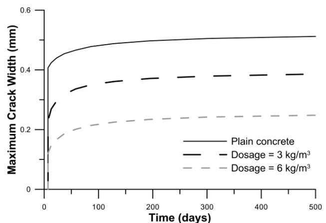
**Fig. 12** Effect of fibre content on the maximum crack width ( $A_{s1} = A_{s2} = 1000 \text{ mm}^2$ ,  $M_e = 100 \text{ kNm}$ ,  $N_e = -300 \text{ kN}$ , creep ratio = 5)
