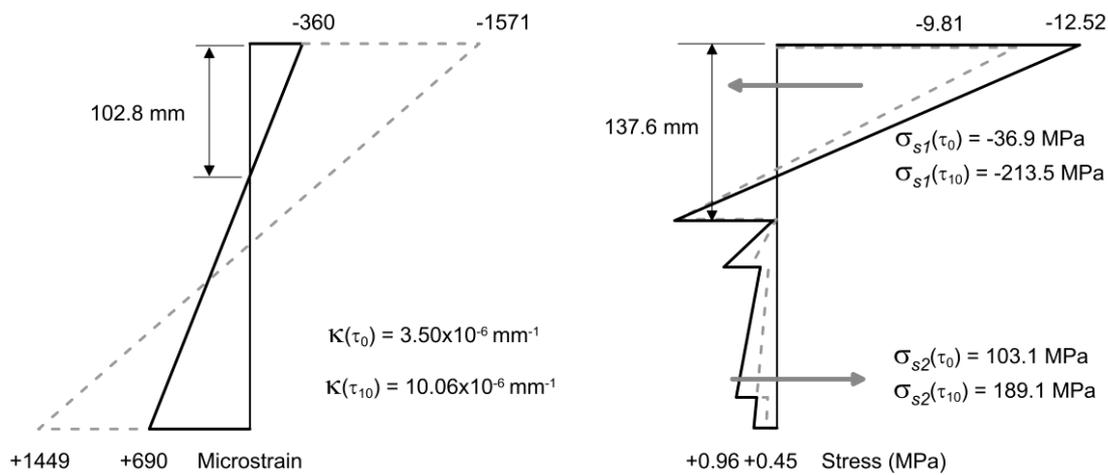
b) Strain and stress distributions for  $N_e = -300$  kN.
