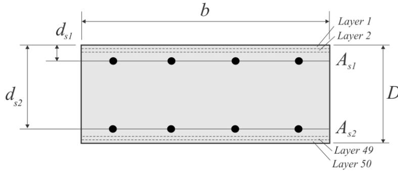
**Fig. 4** Typical layered cross-section containing two levels of reinforcement.
