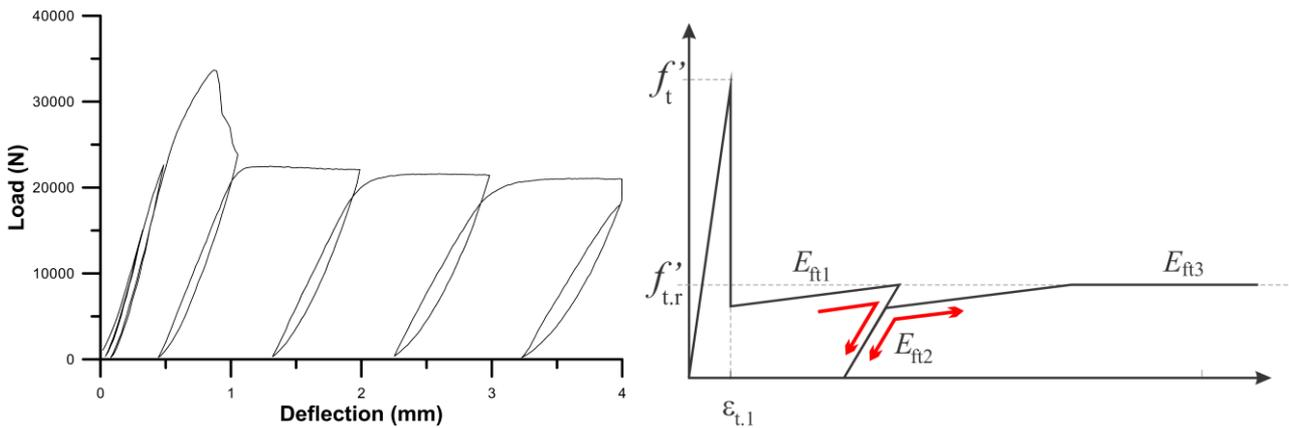
**Fig. 1** a) Test data for macro-synthetic FRC under cyclic loading, and b) idealised stress-strain relation for macro-synthetic fibre-reinforced concrete in tension.
