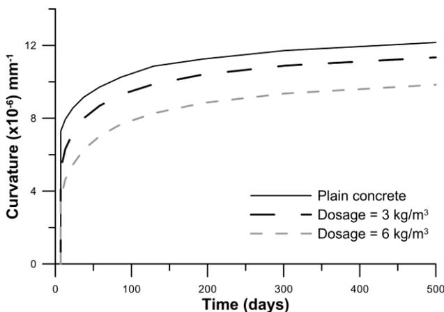
**Fig. 11** Effect of fibre content on the time-varying curvature ( $A_{s1} = A_{s2} = 1000 \text{ mm}^2$ ,  $M_e = 100 \text{ kNm}$ ,  $N_e = -300 \text{ kN}$ , creep ratio = 5)
