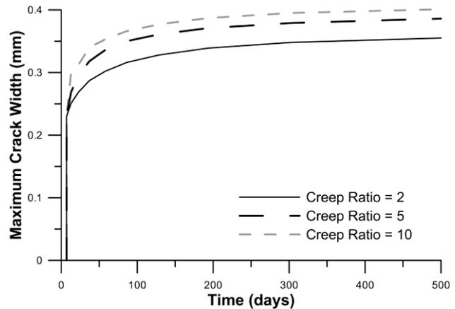
**Fig. 14** Effect of fibre creep on the time-varying maximum crack width ( $A_{s1} = A_{s2} = 1000 \text{ mm}^2$ ,  $\rho_f = 3 \text{ kg/m}^3$ ,  $N_e = -300 \text{ kN}$  and  $M_e = 100 \text{ kNm}$ ).
