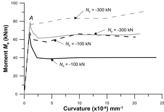
**Fig. 7** Effect of residual tension (fibre content) after cracking on the short-term moment vs curvature relationships for an unreinforced section ( $A_{s1} = A_{s2} = 0$ ).
