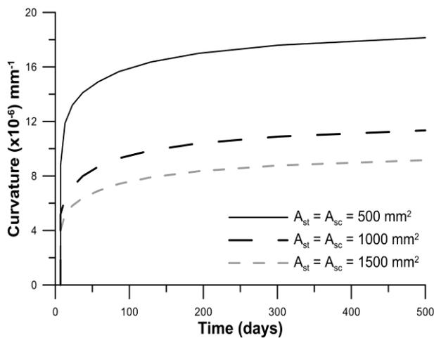
**Fig. 9** Effect of bar reinforcement quantity on the time-varying curvature ( $M_e = 100 \text{ kNm}$ ,  $N_e = -300 \text{ kN}$ ,  $\rho_f = 3 \text{ kg/m}^3$ , creep ratio = 5).
