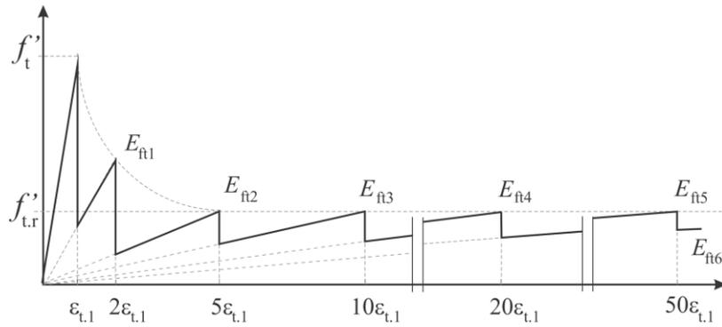
**Fig. 2** Assumed stress-instantaneous strain curve for fibre-reinforced concrete in tension.
