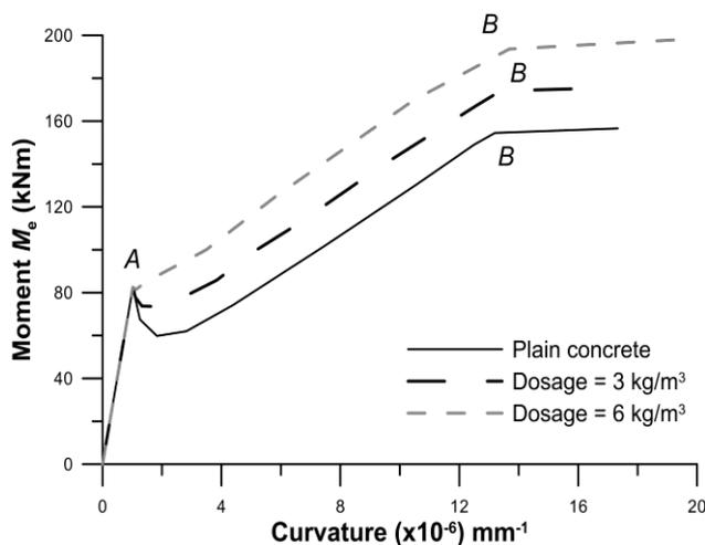
**Fig. 5** Effect of residual tension in fibres after cracking on the short-term moment vs curvature relationships for a section with  $A_{s1} = A_{s2} = 1000 \text{ mm}^2$  and  $N_e = -300 \text{ kN}$ .
