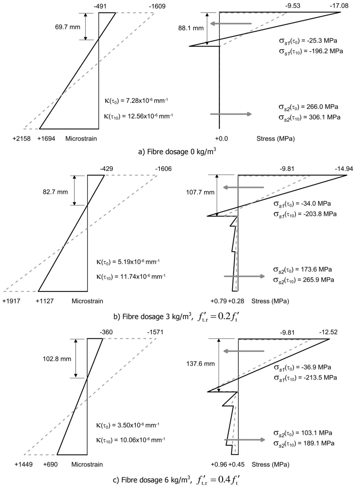
**Fig. 15** Strain and stress distributions on a cracked cross-section at times  $\tau_0$  and  $\tau_{10}$  (with  $A_{s1} = A_{s2} = 1000 \text{ mm}^2$ ;  $M_e = 100 \text{ kNm}$ ;  $N_e = -300 \text{ kN}$ ). Solid lines represent  $\tau_0$  and dashed lines represent  $\tau_{10}$ .
