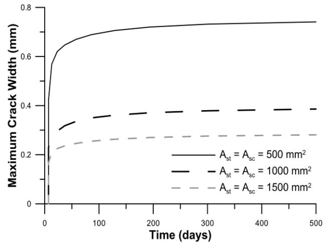
**Fig. 10** Effect of bar reinforcement quantity on the time-varying crack width ( $M_e = 100 \text{ kNm}$ ,  $N_e = -300 \text{ kN}$ ,  $\rho_f = 3 \text{ kg/m}^3$ , creep ratio = 5).
