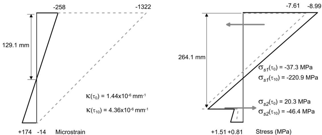
c) Strain and stress distributions for  $N_e = -600$  kN.
