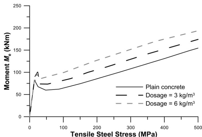
**Fig. 8** Effect of fibre content on the stress in the bottom tensile reinforcement for a section with  $A_{s1} = A_{s2} = 1000 \text{ mm}^2$  and  $N_e = -300$  kN.
