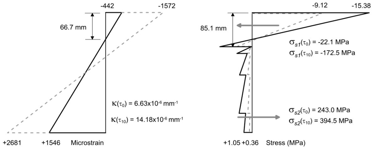
a) Strain and stress distributions for  $N_e = 0$  kN.
