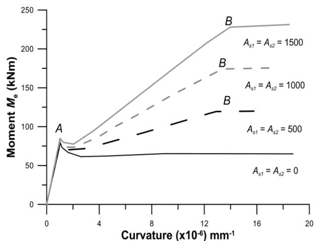
**Fig. 6** Effect of increasing the quantity of tensile reinforcement on the short-term moment vs curvature relationship ( $A_{s1} = A_{s2}$ ,  $N_e = -300 \text{ kN}$ ,  $\rho_f = 3 \text{ kg/m}^3$ )
