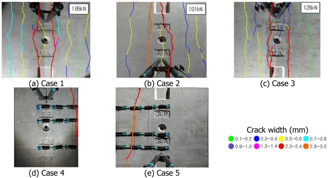
Fig. 10 Crack patterns for each segment specimen at failure
