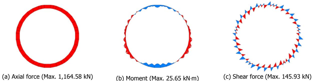
**Fig. 5** Structural member forces in a segment ring
