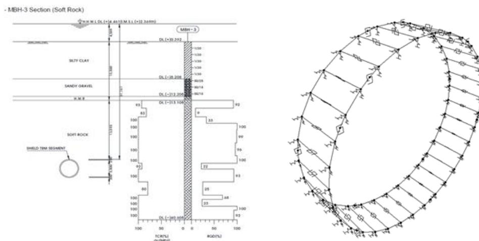
**Fig. 3** Cross-sectional view of a subsea tunnel and its corresponding segment lining model for structural analyses
