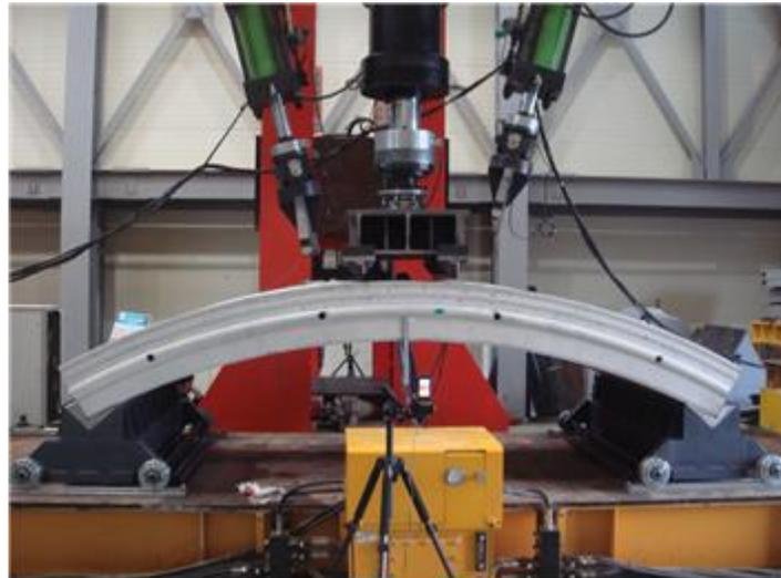
**Fig. 8** Full-scale loading system for a segment
