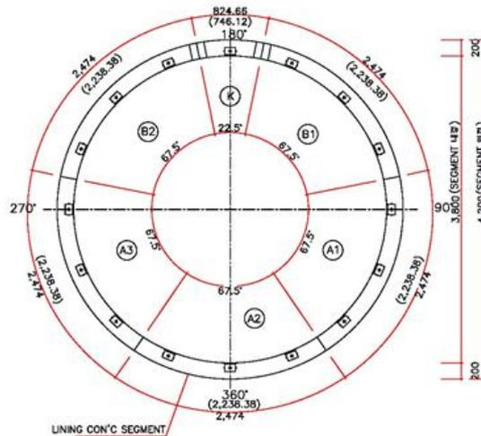
**Fig. 4** Cross-sectional standard drawing of a segment ring in a subsea discharge tunnel
