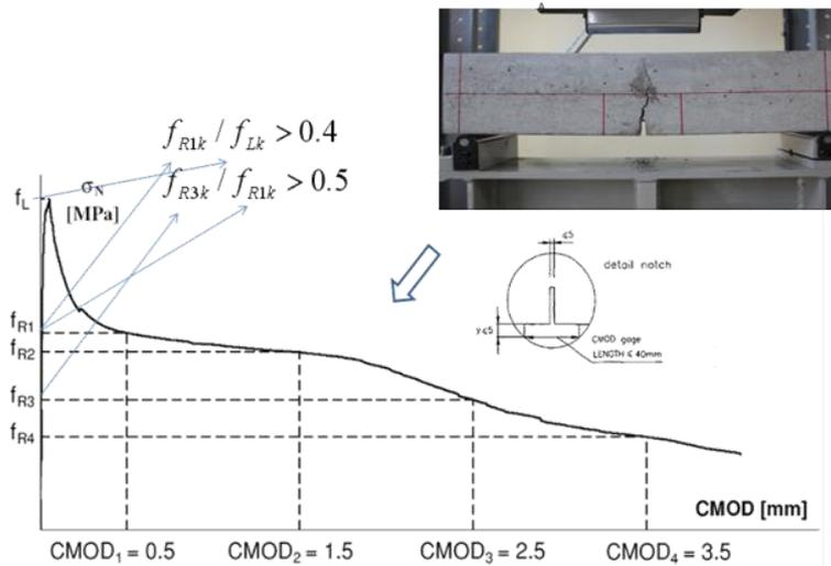
**Fig. 1** Characteristic strengths from a bending test with a notched specimen (FIB, 2010)
