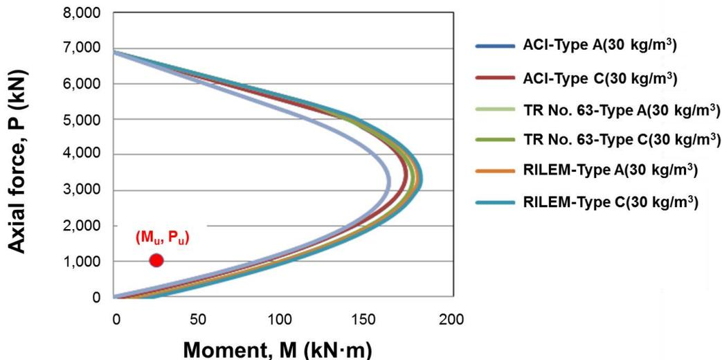
**Fig. 6** P-M diagram of full SFRC segments reinforced with two kinds of steel fibres (dosage: 30 kg/m<sup>3</sup>)
