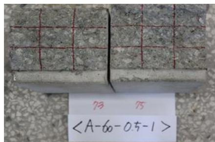
**Fig. 2** Investigation of the number of steel fibres in the ruptured section of a notched bending specimen
