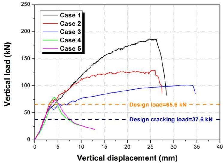
Fig. 9 Load-displacement curves obtained from each segment specimen
