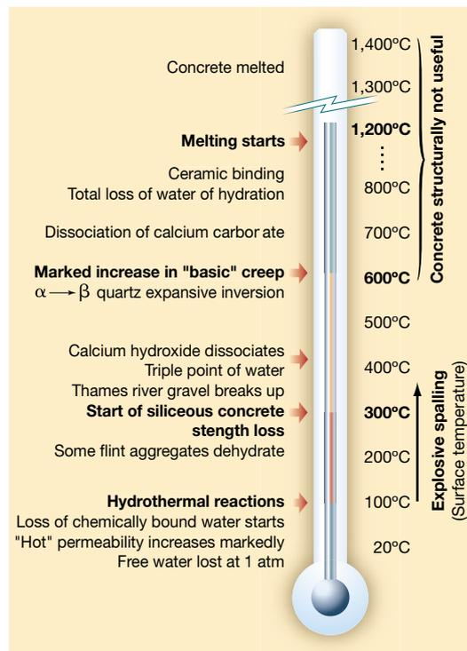
**Top: Fig 2 - Mechanism of spalling of concrete<sup>[2]</sup>**
