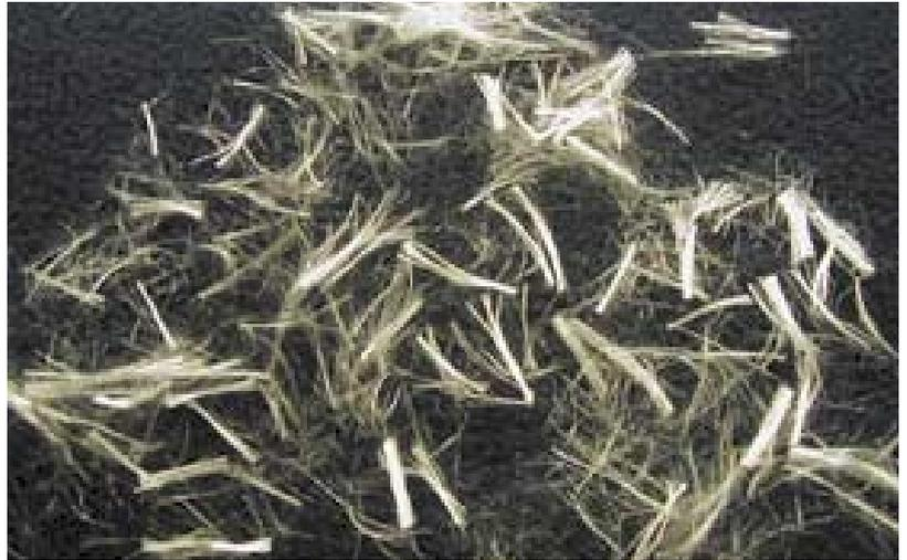
Figure 1: Monofilament polypropylene fibres.
